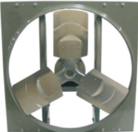
Achieve efficient, economical ventilation in industrial/commercial clean air applications. Fans are shipped assembled and have 2-and 3-wing stamped-aluminum fan blades. Heavy-duty venturi panel, fixed-position motor base with rigid supports. Motors are totally enclosed.
