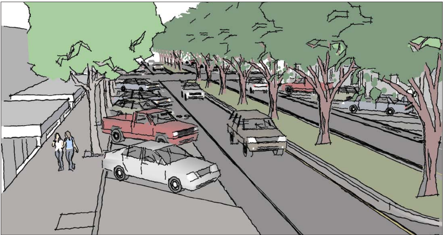
Above: Aerial view of a road diet with reverse-angled parking implemented in the downtown historic commercial core.
