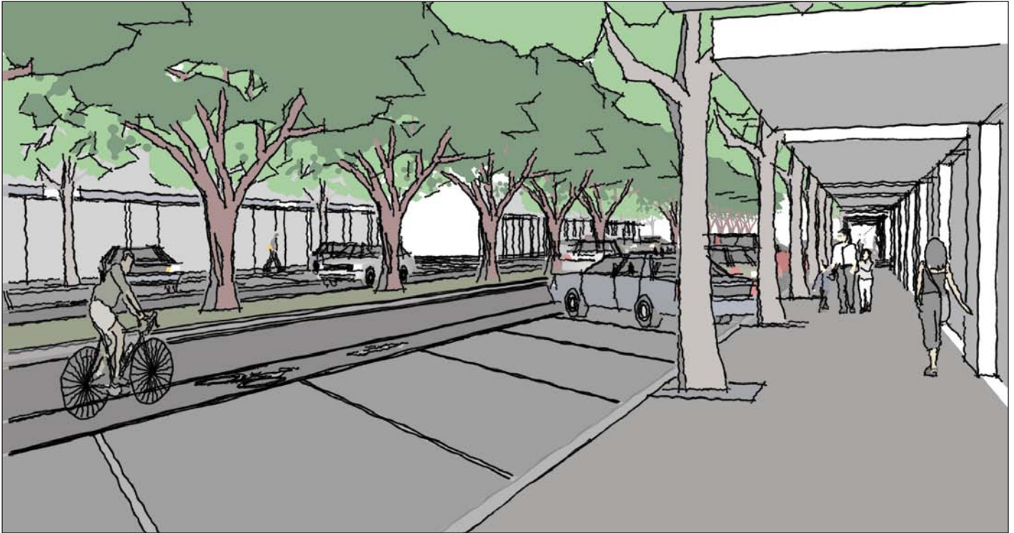
Above: Street view of a road diet with reverse-angled parking implemented in the downtown historic commercial core.
