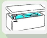
**Step 1** Carefully remove cover from top of toilet tank.
