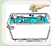
**Step 2** Drop leak detection tablets or food coloring into tank and replace cover.
